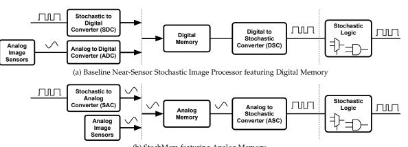
(b) StochMem featuring Analog Memory Fig. 1: Baseline Near-Sensor Stochastic Image Processor vs. StochMem.
