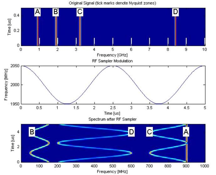
Figure 3: Sinusoid FMCW Sample Clock Signal Example
