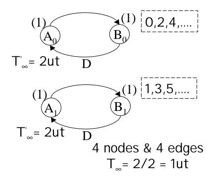
• In a 'J' unfolded system each delay is J-slow => if input to a delay element is the signal x(kJ + m), the output is x((k-1)J + m) = x(kJ + m - J).
